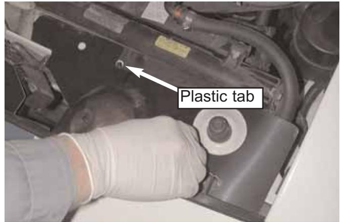
9. Line up the four holes in the nose panel with the plastic tab and the three threaded holes in the bumper support. Doublecheck to make sure that the front edge of the nose panel is not hung up on any phillips headed screws at the front edge of the hood opening.
