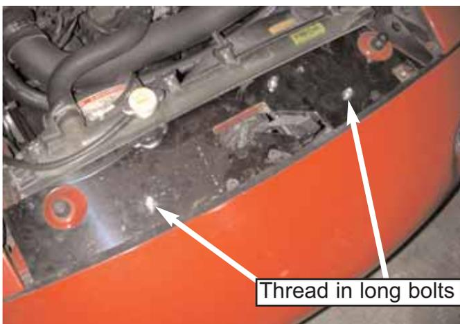
13. Check to make sure that the front edge of the panel is still resting under the rubber hood seal. Then use the 10mm socket, ratchet and extension to hand tighten the three bolts. Do not overtighten!
