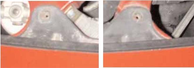
4. Use the 10mm socket, socket extension and ratchet to carefully remove the rearward bolt of the airbag impact sensor. Avoid dropping the bolt into the front nose section. Also avoid dropping the ratchet onto the sensor itself. Place the removed bolt in the same place as the airbag impact sensor cover.
