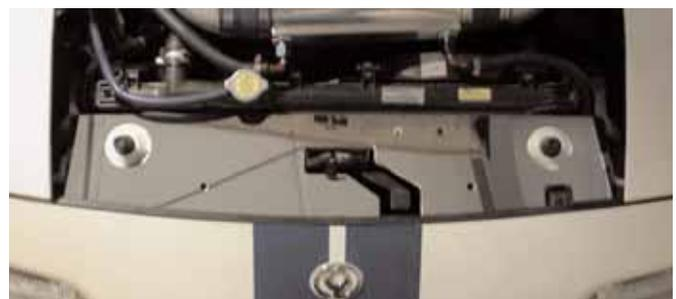
10. If the nose panel holes or washers become misaligned while putting the panel in place, insert the small screwdriver into the hole and move it from side to side or forward and back to adjust the position of the nose panel. Also, the tip of the screwdriver can be used to move the stacked washers back into place.
