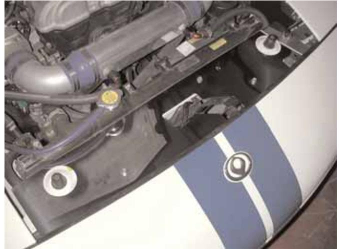
12. Hand thread the two longer bolts included with the kit into the two holes where the washers are stacked. These bolts are both the same length.
