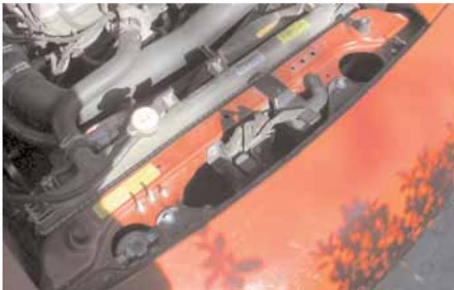
3. Use a 10mm socket, a long extension and the ratchet to remove the two bumper mounting bolts as shown.
